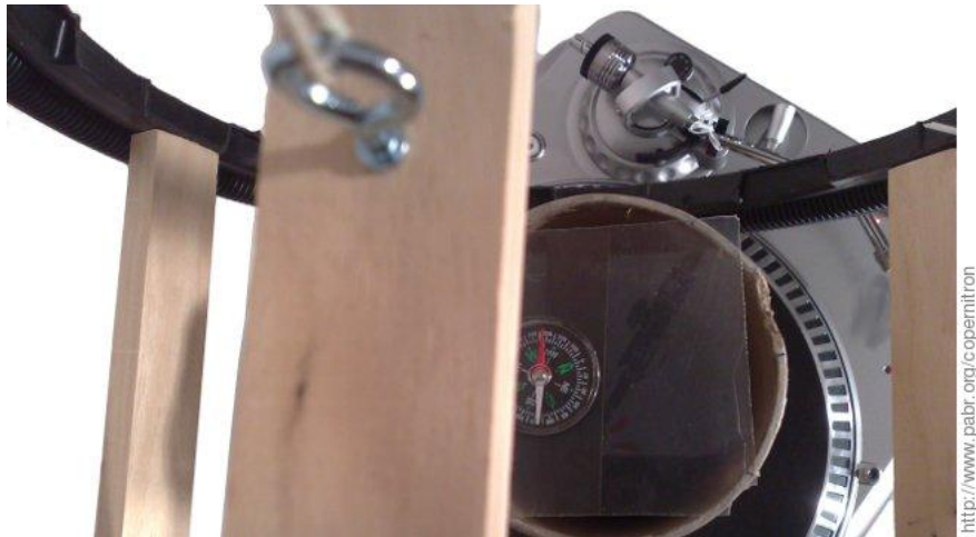
Figure 11. Aligning the inactive coil with Earth's magnetic field
