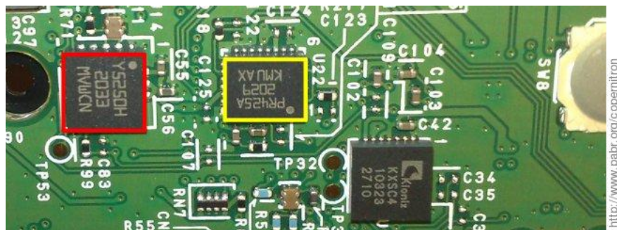
Figure 2. Yaw and Pitch/Roll gyroscopes in a PS Move (CECH-ZCM1E)
